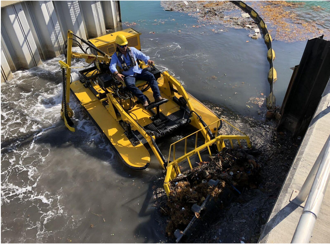
Weedoo shown in operation with loading attachment.
